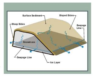
geometry can work to encourage development of sub-basal ice meltwater conduits as the melt season progresses. At this stage, flows across the pad surface are directed along the perimeter of the basal ice (not under or through it). Though the seepages themselves have very low kinetic energy as they exit from the snowfill, erosive power as these flows integrate can become greatly enhanced by the configuration of both the snowfill and the pad on which it is placed.
