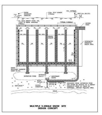
• Construct pad with a single or multiple V-swale configuration (minimum 45m crest-to-crest swale width, 2% side slope to central trough, and 1-2% longitudinal slope).
